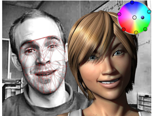
Figure 1: Snapshot of the real-time imitation system. Facial deformations and head movements are captured on the human face (left), and facial deformation are interpreted as a point in the simplified facial expressions space (top right). The virtual character then reproduces the position and the expressive state of the user (right) using its own motion models.
